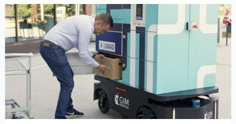
EIT Digital-supported innovation activity Last Mile Autonomous Delivery (LMAD) successfully teamed up with a local supermarket and ran a pilot on the Aalto University Campus near Helsinki. Customers could order groceries online and had them delivered by LMAD's autonomous delivery robot.
